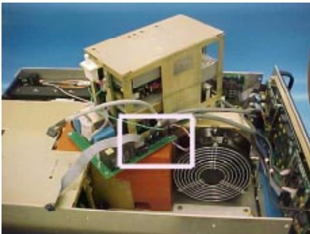
Disconnect the last cables from the PPM as shown at the left to remove the FRU from the HPA
