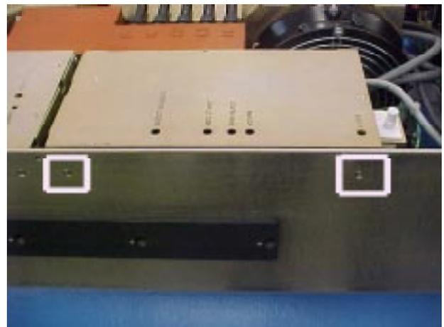
Remove the two-PPM mounting screws from the HPA sidewall (shown at right). The PPC can now be removed.
