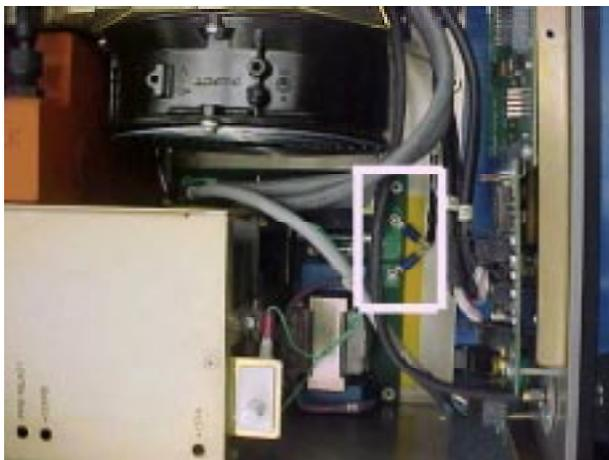
Disconnect the AC wires from the PPM assembly shown at the left.
