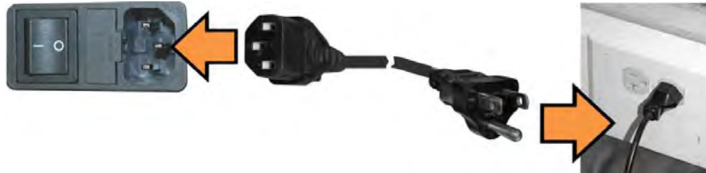
Figure 3-10. Apply AC Power to the CDM-625A
